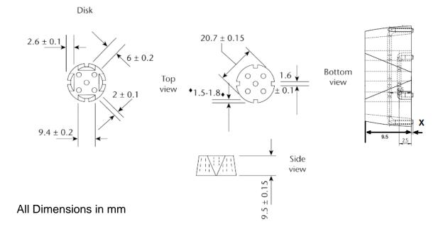
The accuracy of the above mentioned part dimensions have been examined. All relevant measurements are within tolerance and the factory acceptance test has passed. The dimensions are in conformance with USP and Ph.Eur. Pharmacopeia requirements (at time of delivery).
