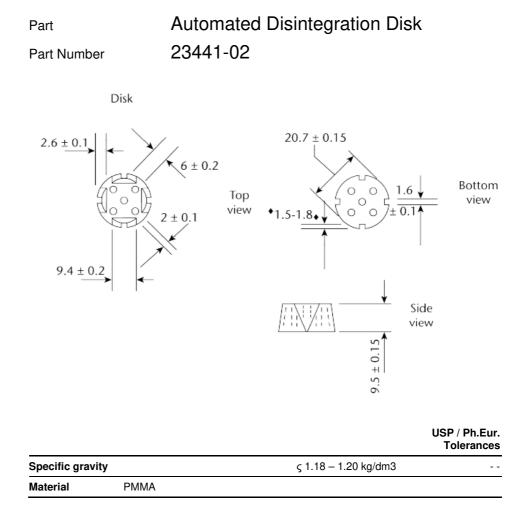
The accuracy of the above mentioned part dimensions have been examined. All relevant measurements are within tolerance and the factory acceptance test has passed. The dimensions are in conformance with USP and Ph. Eur. Pharmacopeia requirements (at date of approval, see below).
