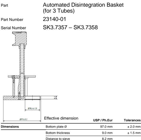
± 2.0 mm ± 1.5 mm Distance to sieve 8.2 mm 3 Holes Ø 38.3 mm ± 2.3 mm PMMA, POM, PVC, PA Material
