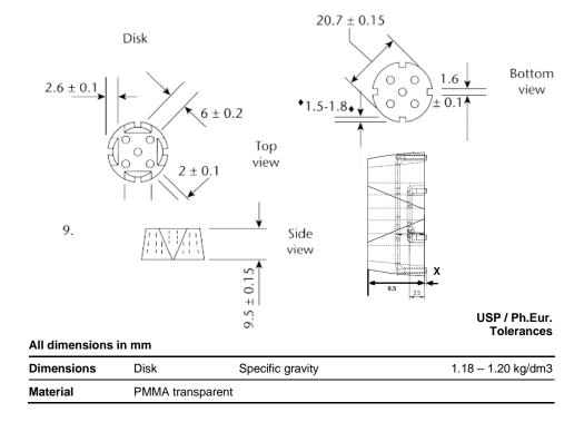
The accuracy of the above mentioned part dimensions have been examined. All relevant measurements are within tolerance and the factory acceptance test has passed. The dimensions are in conformance with USP and Ph. Eur. Pharmacopeia requirements (at date of approval, see below).
