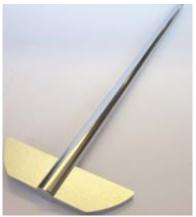
Tolerances Dimensions: Paddle Height 19.0 mm ± 0.5 mm Upper length 74.5 mm ± 0.5 mm Lower length 42.0 mm ± 1.0 mm Size 4.0 mm ± 1.0 mm Radius 1.2 mm ± 0.2 mm Radius 41.5 mm ± 1.0 mm Shaft Diameter 9.4 to 10.1 mm
