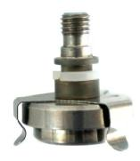
Dimensions: Cap  $\varnothing$  25.0 mm  $\pm$  3.0 mm Cap size 5.1 mm  $\pm$  0.5 mm Clear opening 20.2 mm  $\pm$  1.0 mm Vent hole  $\varnothing$  2.0 mm  $\pm$  0.5 mm
